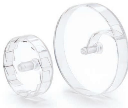
Pic.: Friability (right) and abrasion (left) drum
